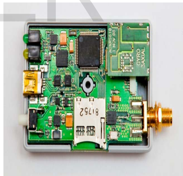
Fig-2, Flexible wireless ECG sensor with a fully functional microcontroller. Developments in the field of flexible electronics are expected to lead to the advent of smaller, lighter and more comfortable wearable systems.
